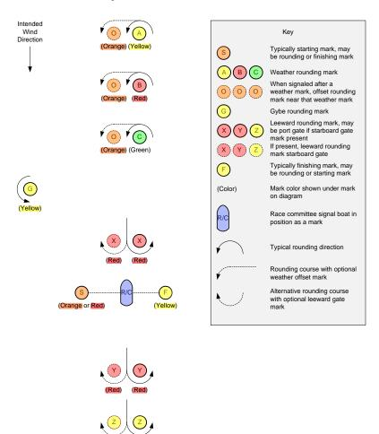
The course diagram for buoy course marks shows the general orientation of the race committee signal boat ("R/C"), other marks (identified by the letters S, A, B, C, O, G, X, Y, Z and F), and the intended wind direction. All marks other than the race committee signal boat are inflatable buoys. Positions are approximate and the diagram is not to scale.
